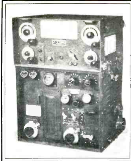
This behemoth was intended for use in the "Betty" medium bomber. The 6-tube receiver is at the top. Below is the 20-watt AM/CW/MCW 2-channel transmitter. It operated between 220 kHz and 10 MHz in two bands. Was rated for 200 mile CW range at 10,000 ft.
