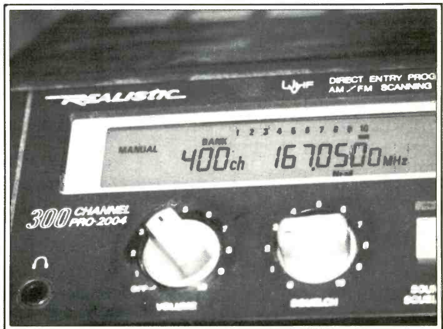
Note that this modified PRO-2004 shows it receiving on Channel #400. Not bad for a scanner that was only supposed to receive 300 channels! You may not even be able to fill up all 400 channels with active frequencies.
